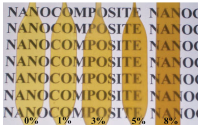
Figure 8 Photograph of ESO40-organoclay nanocomposites with 1–8 wt % OTAC. [Color figure can be viewed in the online issue, which is available at www.interscience.wiley.com .]
